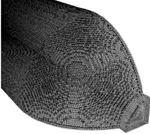
Figure 2: 3D plot of the CFD grid of the floating head.
