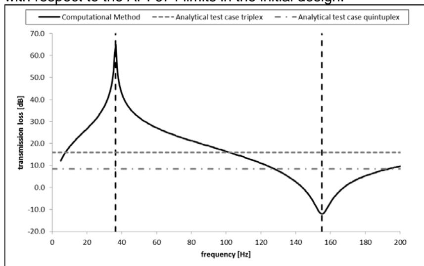
Figure 5 | Typical transmission loss profile branch connected accumulator.
