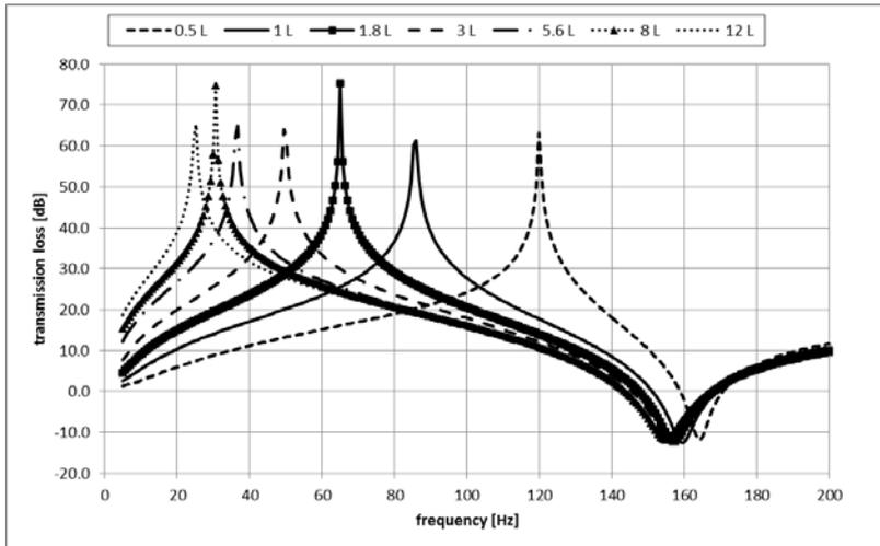
Figure 6 | Transmission loss for branch type accumulator with different gas volumes.
