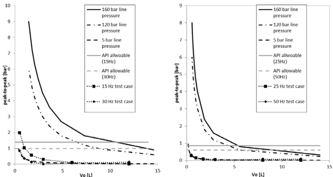
Figure 4 | Comparison predicted initial peak-to-peak pulsations analytical method and computational method with API limits, Triplex pump (left), quintuplex pump (right).
