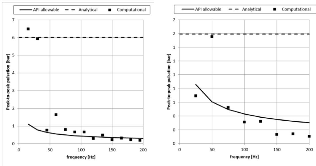
Figure 3 | Initial peak-to-peak pressure pulsation frequency spectrum. Triplex (left), Quintuplex (right).
